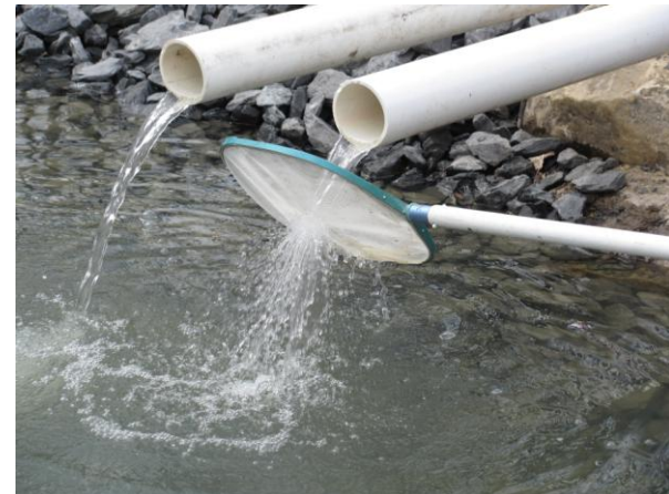
Window screens to increase the agitation thereby increasing DO
